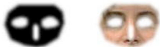
Figure 4: Mask used to estimate the global warp. Each image is warped to account for changes in the head’s position, size, and rotation. The transform minimizes the difference between the transformed images and the face template. The mask (left) forces the minimization to consider only the upper face (right).
